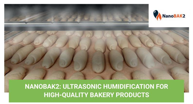
The project's aim is to test and disseminate the technical feasibility and economic viability of UltraBAK technology, an efficient **ultrasonic humidification system** for **bakery** cooling and fermentation processes.
